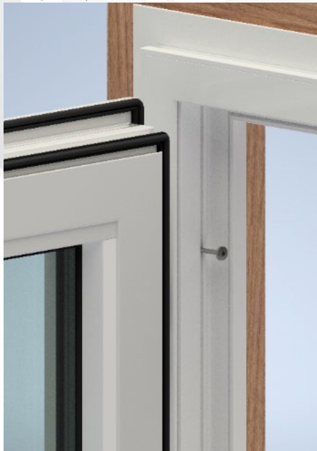
Figure 15: Partially Fastened Jamb Fastener
