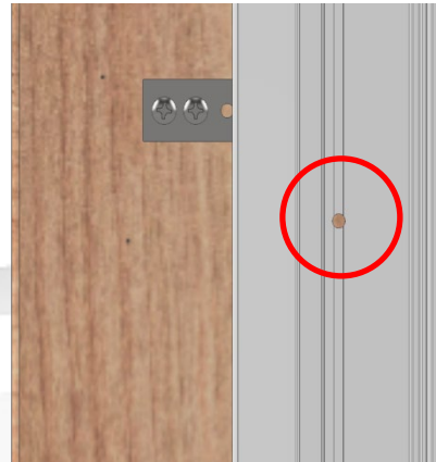
Figure 14: Revealed Jamb Fastening Pilot Holes
