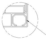
DETAIL C SCALE 1 / 2 FRAMES REINFORCEMENT INSTALLED IN FRAMES LARGER THAN 36" IN WIDTH TOLERAN DECIMA  $X.X \pm 0.1$   $X.XX \pm 0.0$   $X.XXX \pm 0.0$ FRACTIO  $X/X \pm 1/32$  $\frac{\text{ANGULAR}}{\text{X} \pm 1.0}$   $\text{X.X} \pm 0.2$
