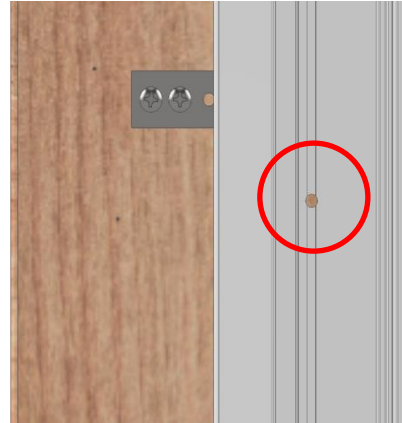
Figure 14: Revealed Jamb Fastening Pilot Holes
