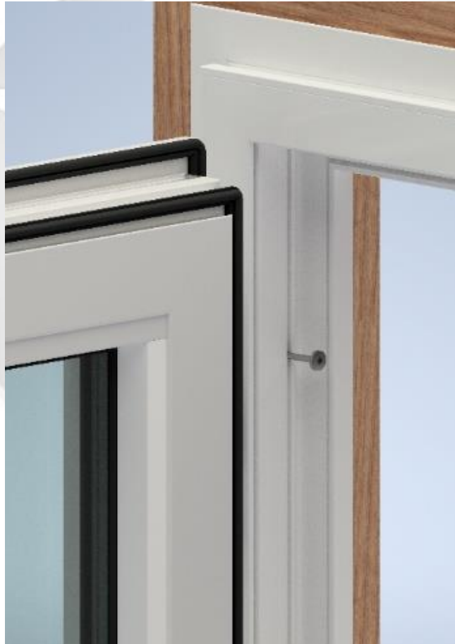
Figure 15: Partially Fastened Jamb Fastener
